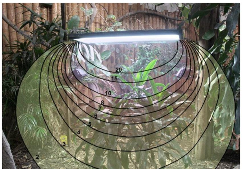
Fig. 8. The UVI gradient beneath an 8-tube installation at Chester Zoo
