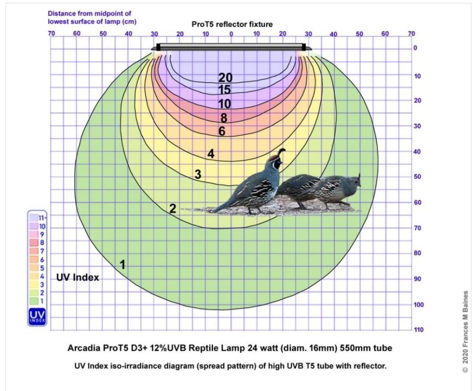
Fig. 7. The UVI gradient beneath a typical T5-HO UVB lamp
